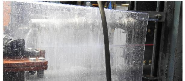
Fig. 18. Quenching unit designed and manufactured by the community for the simulation of DQ and DQ&P.
