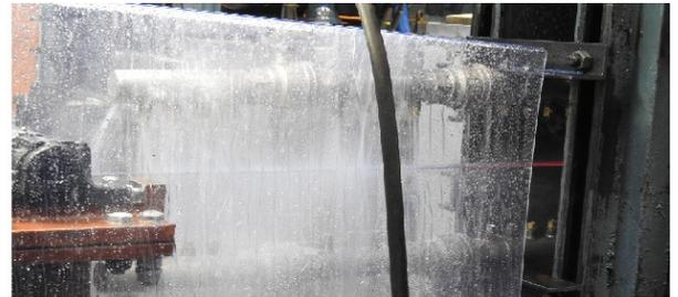
Fig. 18. Quenching unit designed and manufactured by the community for the simulation of DQ and DQ&P.
