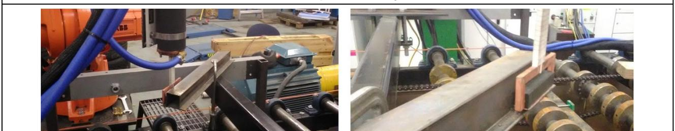
**Fig. 9. The updated MP25 unit (capacitor tank + inductors) showing a coil for annealing outer corners (welded structures) as an example.**
