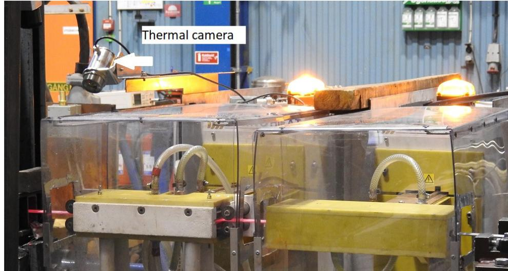
Fig. 17. Quenching unit designed and manufactured by the community for direct quenching (DQ) and direct quenching and partitioning (DQ&P) processes.
