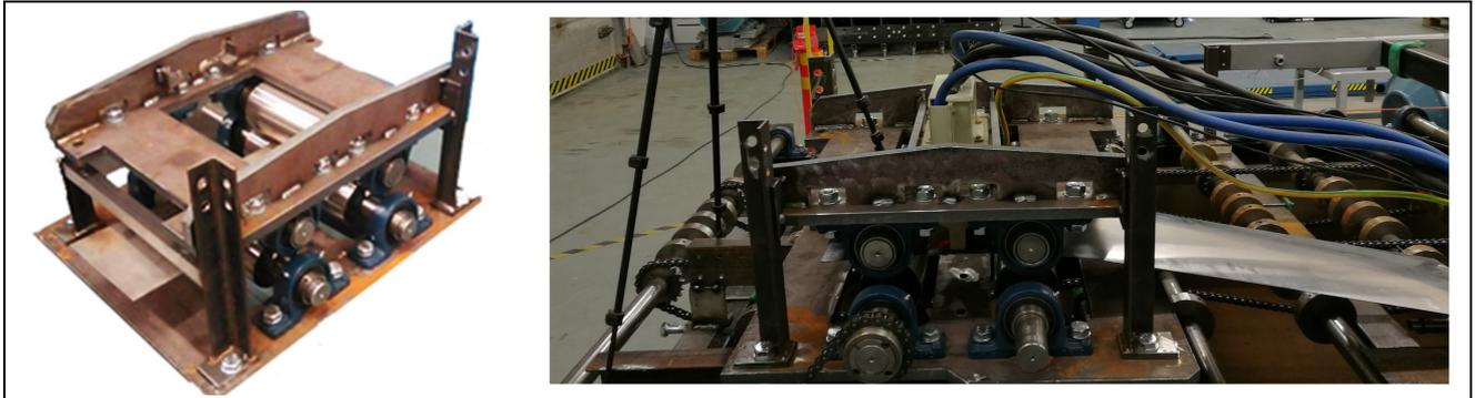
**Fig. 6. Sheet support system for the MP25 “knife inductor”.**
