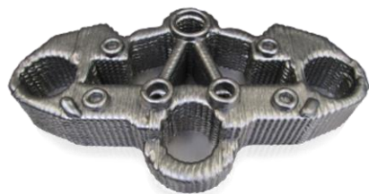
Printed Blank (6.5 h) 25 kg (printed volume: 17 kg)
