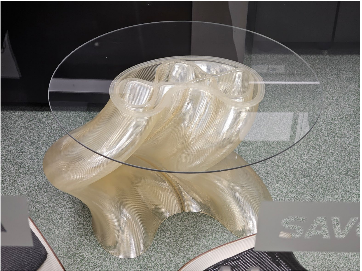
Figure 2. Table frame was designed to be printable with one continuous loop
