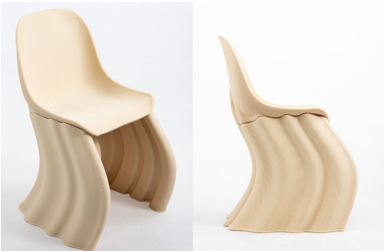
Figure 6. Chair printed with KCL biocomposite
