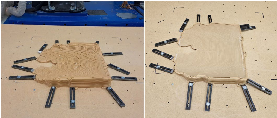
Figure 1. 3D-printed mold of the seat after printing and after milling
