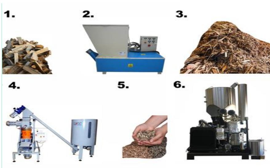
1. Biomass is fed into shredder. 2. Shredder produces biomass stock. 3. The biomass stock that is fed into pelletizer to produce pellets. 5. The pellets are fed into hopper container. 6. The gasifier produces syngas from pellets.
