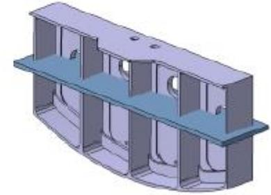
(d) Plane of Symmetry or Partial Symmetry (Not Aligned with a Wall)
