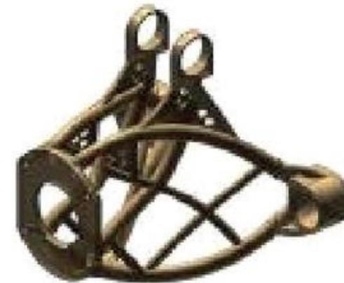
b) Modified result design by topological optimization and produced by PBF-LB/M
