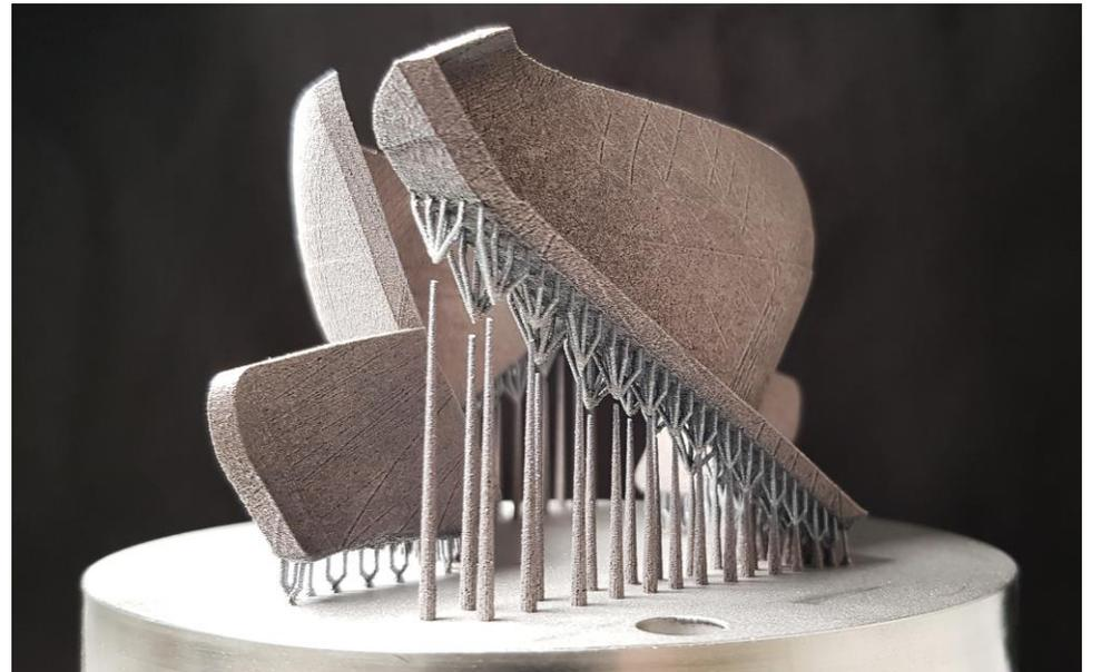
Printed test pieces – to evaluate material quality and distortion of printed parts (input for simulations)
