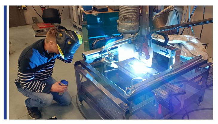
3D printing of metals by direct layering is possible with modern robotic welding cells and CNC mechanized solutions that are used in industry. The goal of the project is to promote the renewal of the engineering industry in the region by utilizing already existing equipment for the direct deposition of metals.
